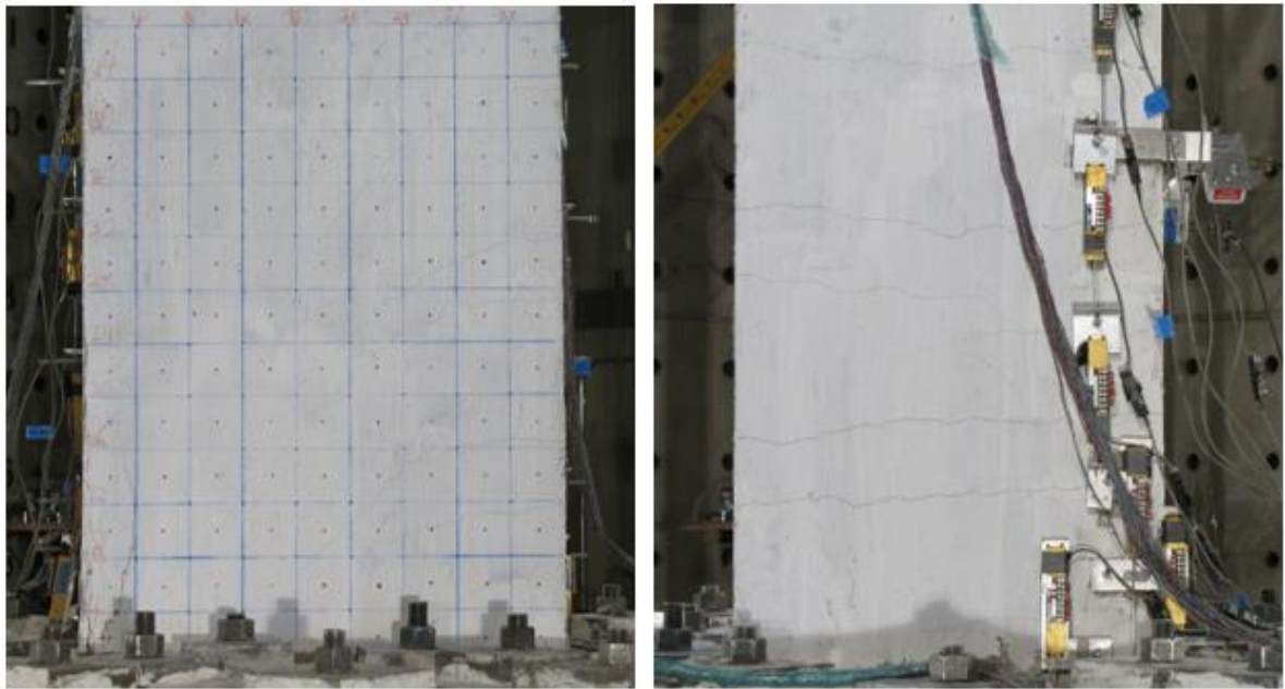
Figure 12. Column condition for 3rd set of MIRA measurements (after 1% drift ratio was attained).
