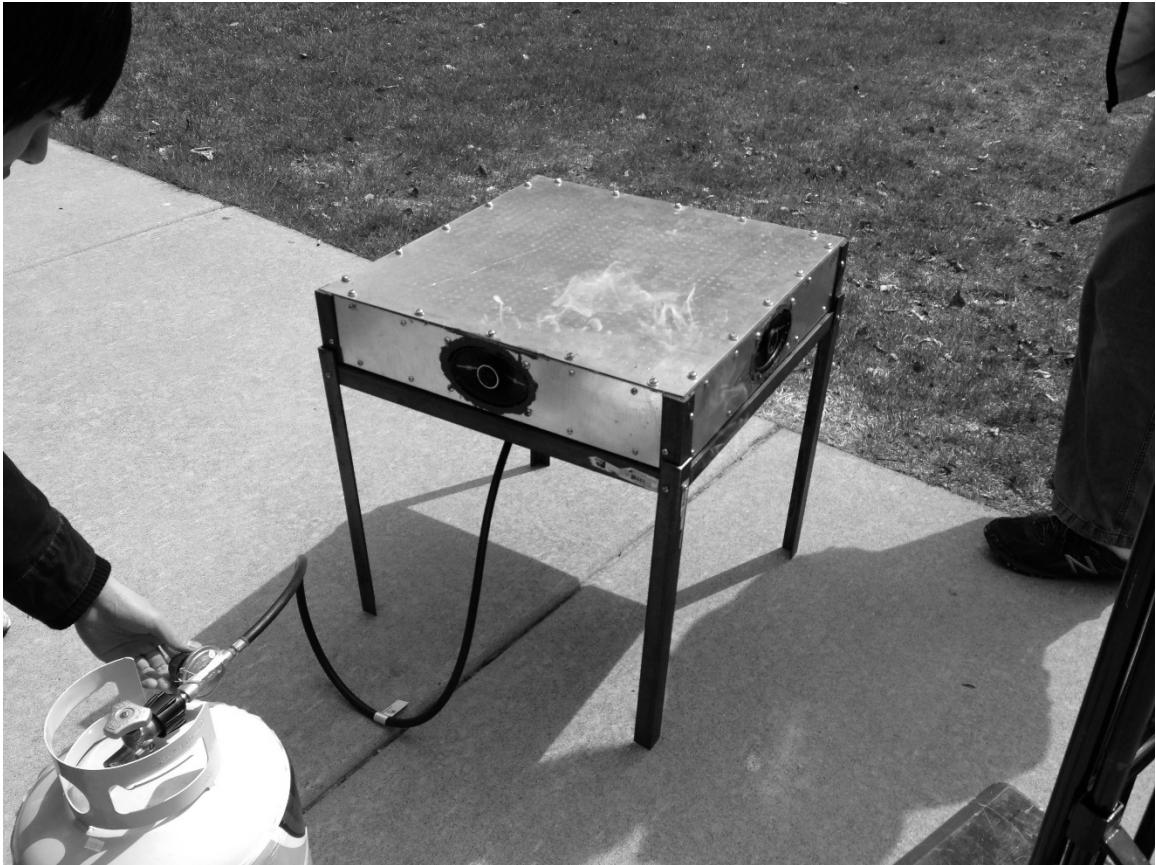
Figure 8: The Pyroboard, Version 2, a Fire Generating Device that "Dances" to Music
