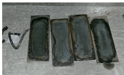
Figure B.3 Photographs of CZTS nanocrystal coatings on Mo foil after deposition of 70 \mu\text{L} of Se-containing ethanethiol and ethylenediamine solution on top of coating. A significant amount of residual carbon was as the solution dried.
