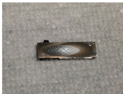
Figure 6.2 Photograph of CZTS nanocrystal coating after annealing using “hot-loading” method where furnace was preheated to 600 °C before inserting the annealing ampule with the coating. The plume region is likely caused by sulfur condensation on the thick Mo-coated SLG substrate due to uneven heating.
