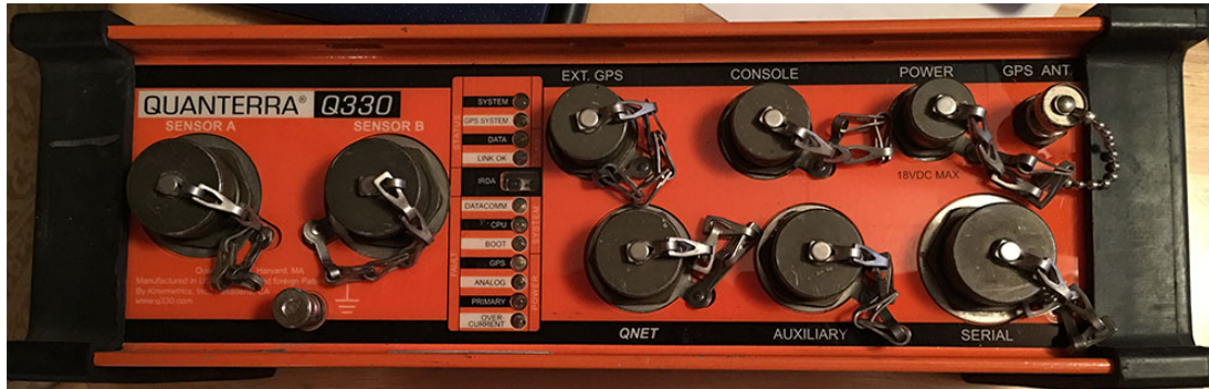
Figure 6.2: Photo of a Quanterra Q330 datalogger. The seismometer is connected through one of the SENSOR ports on the left. A GPS antenna may be connected to the GPS ANT port or an external GPS source may be connected to the EXT GPS port. The Q330 is connected to a Baler via the SERIAL port and/or to a local network through the QNET port. The Q330 is powered either via the POWER port or through the QNET port. All connections (other than GPS ANT) are military-type; more details can be found in the Q330 manual [326].
