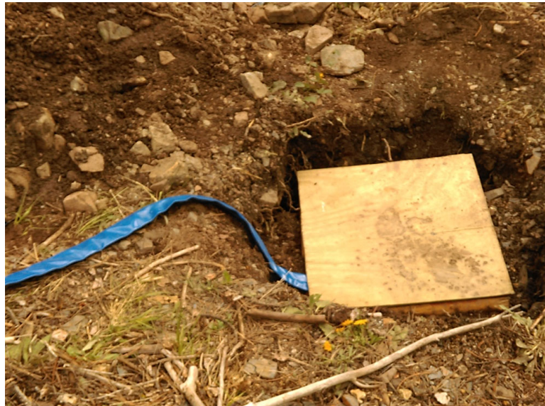
Figure 6.5: Seismometer vault at TPK surface station, sealed with plywood. The seismometer cable is inside of the blue conduit.
