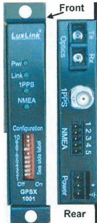
Figure 6.12: Front and rear views of a GPS transceiver. The 1PPS and NMEA lights blink when receiving the corresponding signal. The optical signal is input through the Rx port and is output from the Tx port. The electrical 1 PPS and NMEA signals are output (or input, depending on dip switch settings) through the BNC jack and the terminal block, respectively.
