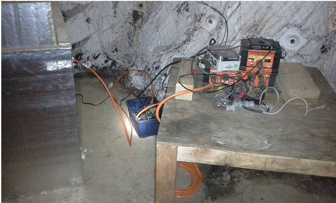
Figure 6.8: Data acquisition system and electronics for the underground sites (B4850 station shown here). The Q330 and Baler are shown on a wooden table along with a power box (on top of Q330, to left of Baler) and a GPS transceiver (small black object on top of Baler). The battery is in the purple tub on the ground.
