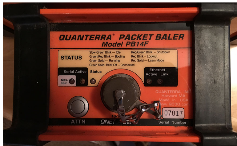
Figure 6.3: Photo of a Quanterra PB14 Packet Baler. The Baler is connected to a Q330 via the QNET + SERIAL port and receives its power through this connection. The ATTN button is used to “wake” the Baler from its low-power state; when the Baler has completed its boot cycle, the Q330 it is connected to will automatically begin transferring data to it.
