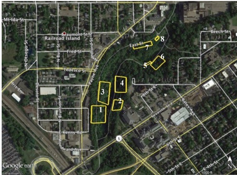
Figure 13: Proposed survey areas based on historic map overlays and GPR.
