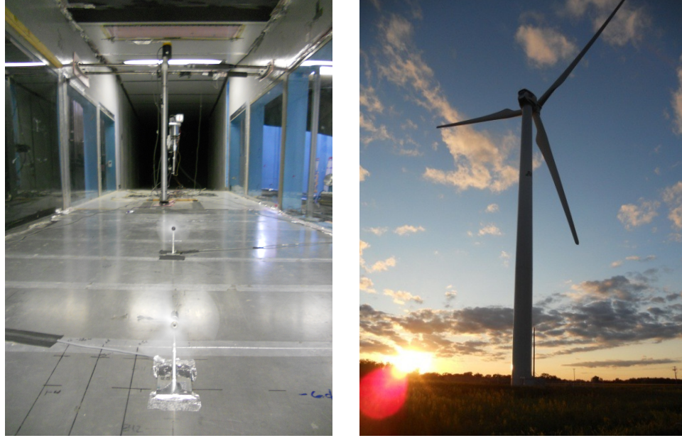
Figure 3.2: Two turbine setup in the SAFL wind tunnel (left) and the 2.5 MW Clipper turbine at UMore Park (right). Photo credit: Kevin Howard.
