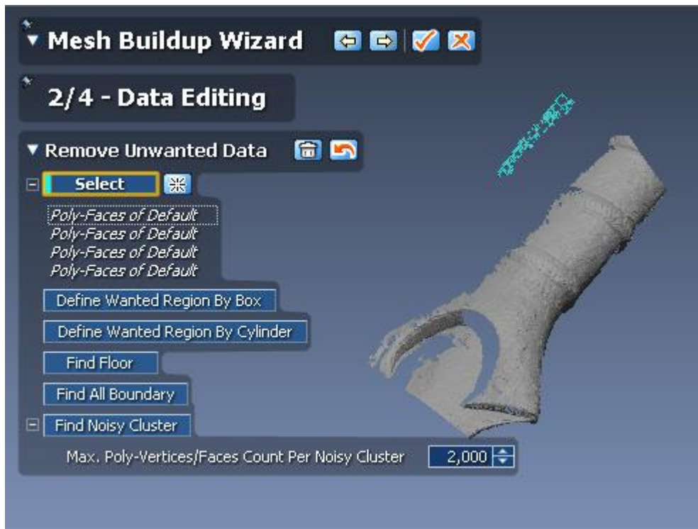
Figure A.8: Removal of remaining extraneous data for sword 10.048.
