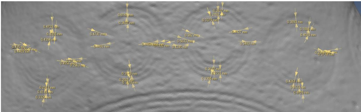
Figure A.21: Diameter, distance between centers, and distance between circles for concentric circle measurements on hilt 9.201.
