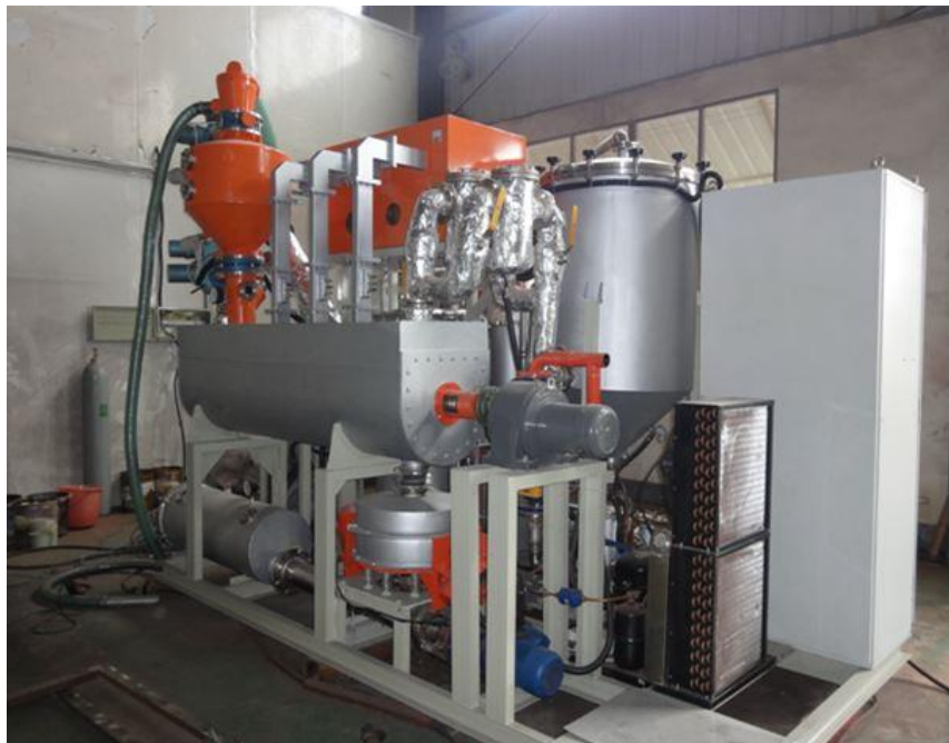
Figure 4.2. Photo of a mobile microwave assisted pyrolysis (MAP) unit. This unit can be put on a trailer and moved with a pick-up truck. Dimensions are approximately 5.0 x 2.5 x 3.5 meters.
