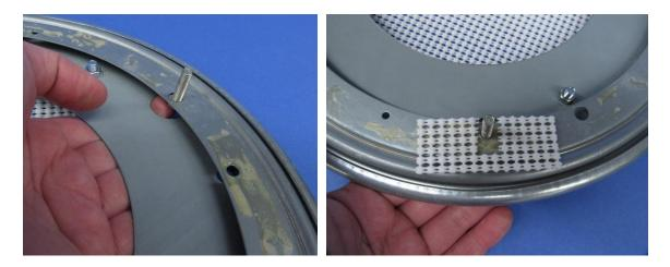
Attach the connector to the lazy susan bearing using the center screw and a nut.
