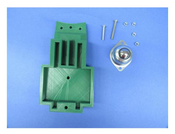
Insert the 30 mm screw through the hole in the center of the arm mount and the 40 mm screw through the hole in the end of the arm mount. Depending on the exact height of your feet, you may need to add nuts or washers on the back of the arm mount to act as spacers so the mount sits level on the lazy susan bearing. Here, I've used two nuts attached to the screws on the bottom of the arm mount as spacers.
