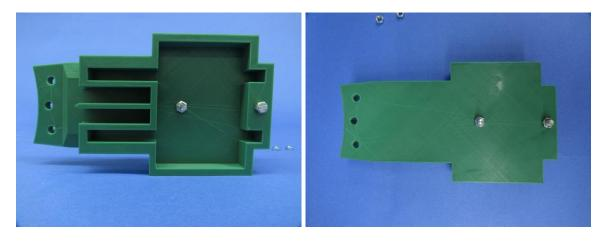
Position the 1" roller ball transfer bearing over your screws, and secure with nuts.
