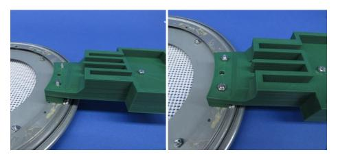
Set the 3D printed platform base in the center of the lazy susan bearing on top of the shelf liner. Put another piece of shelf liner cut to fit the top of the platform base on top of that.
