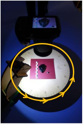
Move the flashlight down to the 50 degree mark on the rig arm. Move the rig arm so that it is centered around the 15 degree mark on the rig platform. Take a photo, move the arm 30 degrees to the 45 degree mark on the platform, and take another photo. Continue this pattern moving around the platform and moving the flashlight down in 10 degree increments down the rig arm after each rotation. A table of the lighting positions I usually use are listed on the following page.
