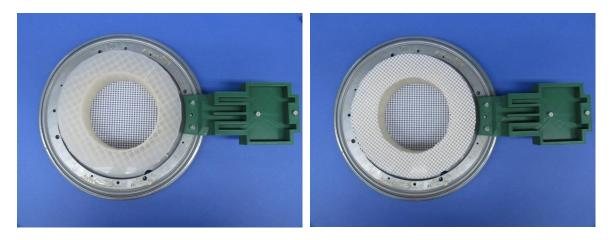
Place the laser cut platform on top of the platform base. Make sure it is centered, and that the arm mount can rotate freely around the entire perimeter of the platform.
