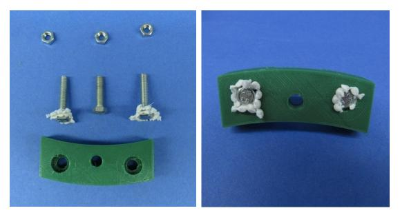
There should be a hole in the bottom of the bearing that allows you to stick a screw through the top. Push a 20 mm screw through this hole. In order to prevent the connector from shifting once the rig is assembled, lay a piece of shelf liner across the top of the bearing.
