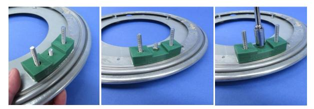
3. Attach the 1" roller ball transfer bearing to the bottom of the 3D printed arm mount. You will need the arm mount, bearing, one 30 mm long screw, one 40 mm long screw, and nuts / washers / spacers (optional).
