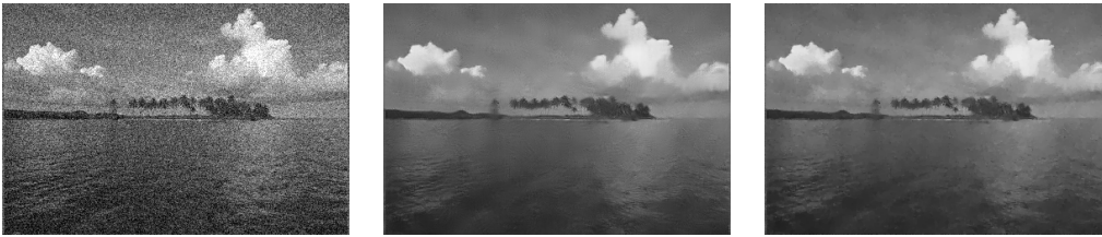
FIG. 3.3. Left: noisy image. Middle: result obtained with NLM denoising of the image. Right: result obtained with NLM denoising of the curvature image.
