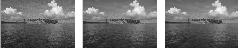
FIG. 1.4. Left: noisy image I . Middle: the result \hat{u} obtained with (1.2). Right: original clean image a .
