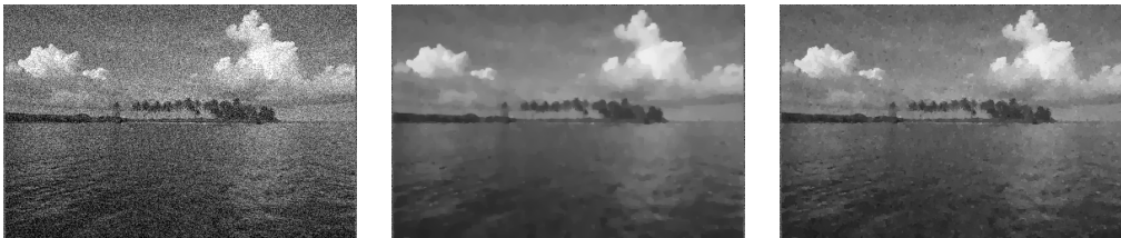
FIG. 3.1. Left: noisy image. Middle: result obtained with TV denoising of the image. Right: result obtained with TV denoising of the curvature image.
