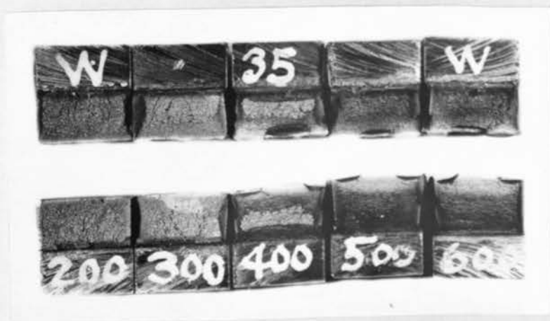
b. Fractures of representative series W specimens S.A.E. 1035 steel.
