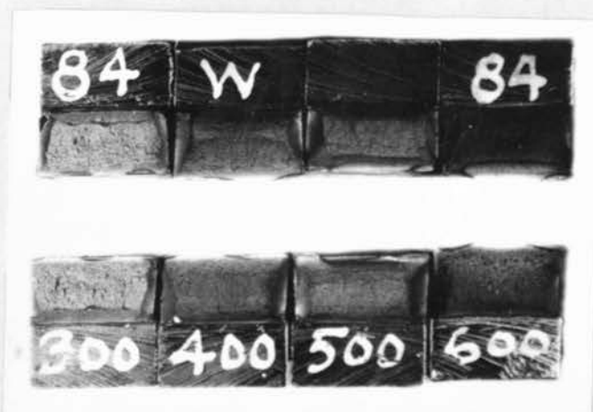
b. Fractures of representative series W specimens S.A.E. 3140 steel.
