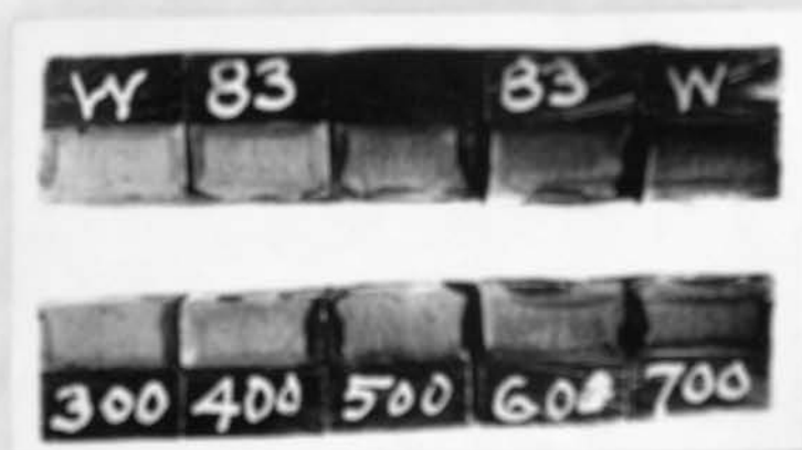
b. Fractures of representative series Y specimens B.A.S. 3130 steel.
