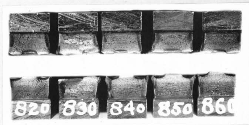
a. Fractures of temperature test specimens S.A.E. 1035 steel. Temperatures marked on lower halves of specimens.
