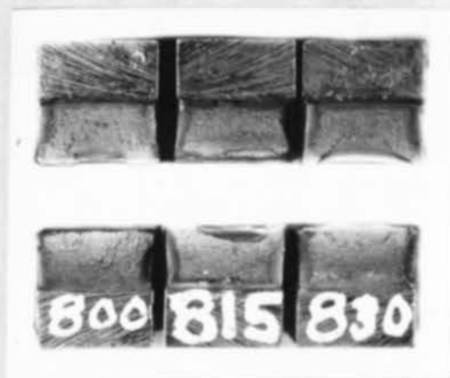
a. Fractures of temperature test specimens S.A.E. 3130 steel.
