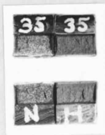
a. Fractures of hardened(H) and normalized(N) specimens S.A.E. 1035 steel.
