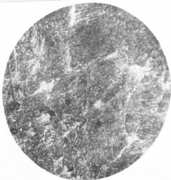
b. Microstructure:specimen 35-4. X 1000. Troostite with original ferrite.
