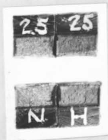
b. Fractures of hardened and normalized spec- imens S.A.E. 1025 steel.
