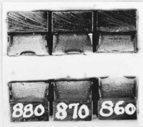
a. Temperature test specimens S.A.E. 3120 steel.
