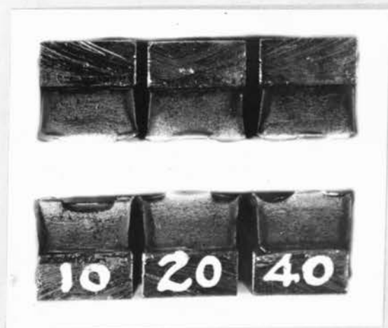
b. Fractures of time test specimens S.A.E. 1035 steel. Times marked on lower halves.
