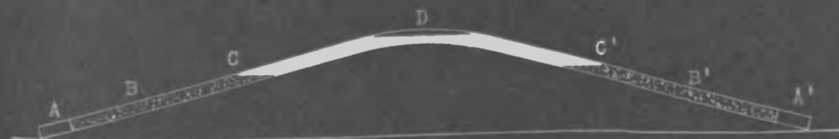
Fig. 14. GLASS TUBE SHOWING THE RESULTS OF FORTY EIGHT HOURS' ACTION ON TUBE AS SHOWN IN FIG. 13. A AND A', DOLOMITE; B AND B' SEA WATER IN SAND; C AND C' SEG- REGATION OF OIL IN THE SAND; D, ACCUMULATION OF GAS IN SAND.
