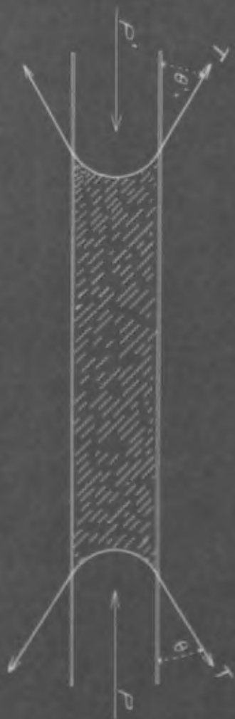
Fig. 11. MENISCUSES FORMED BY A DROP OF A LIQUID IN A CAPILLARY TUBE.
