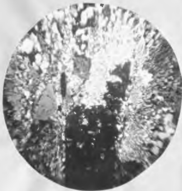
B. Micropegmatite Around Euhedral Plagioclase
