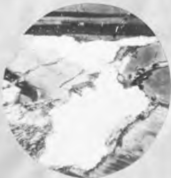
D. Fractured Plagioclase Beside Unfractured Quartz
