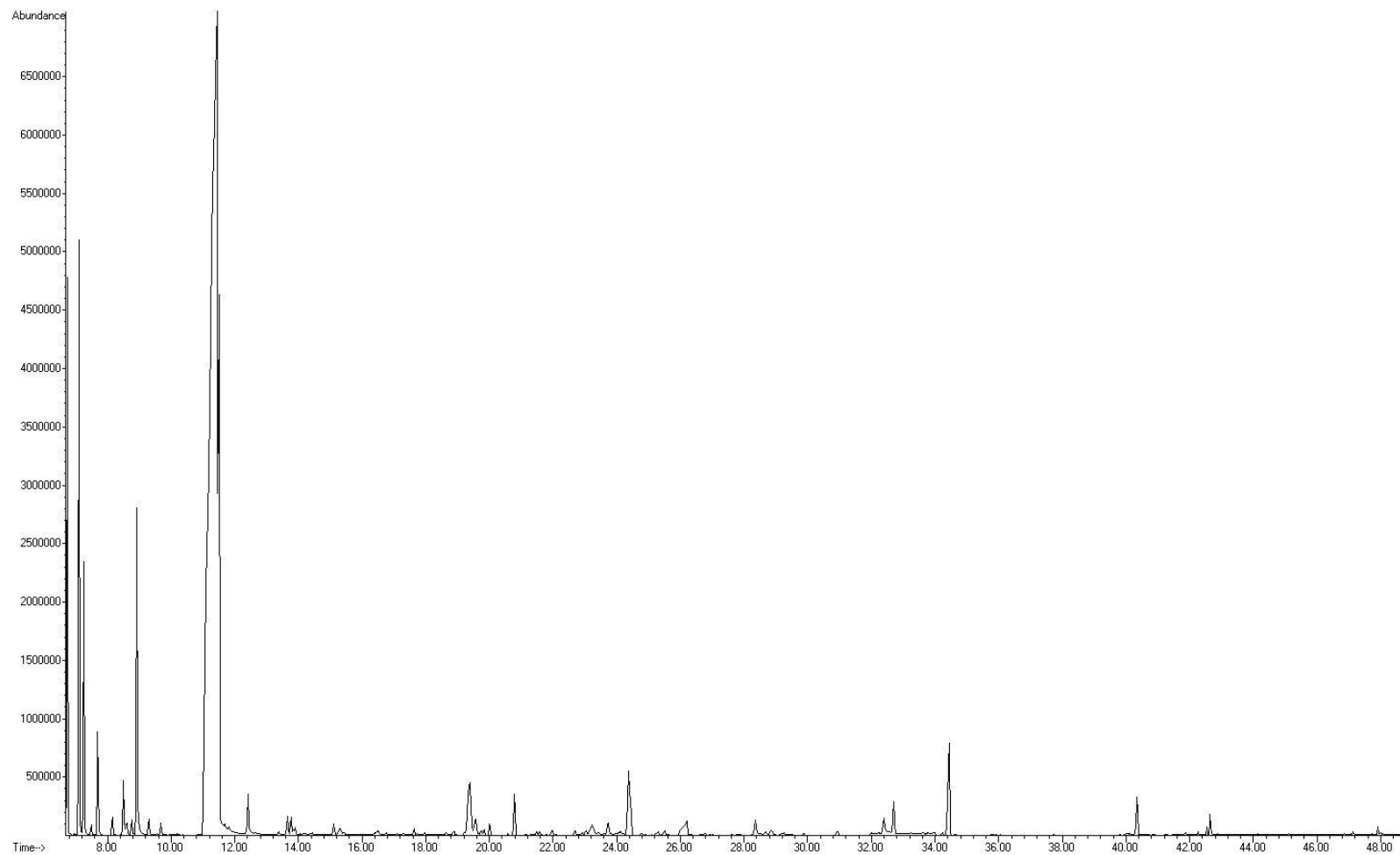
Figure 21. Whole wheat bread crust extract chromatogram SIM DB-5 column
