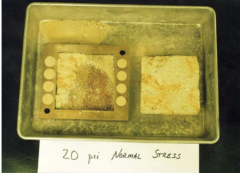
Figure 3-13: St. Peter sandstone sheared at 152 kPa normal stress. The photo shows diminished topographic relief.
