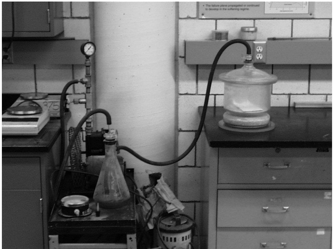
Figure 4-1: Vacuum apparatus used to evacuate the impregnating resin and the pore space in the St. Peter sandstone samples.
