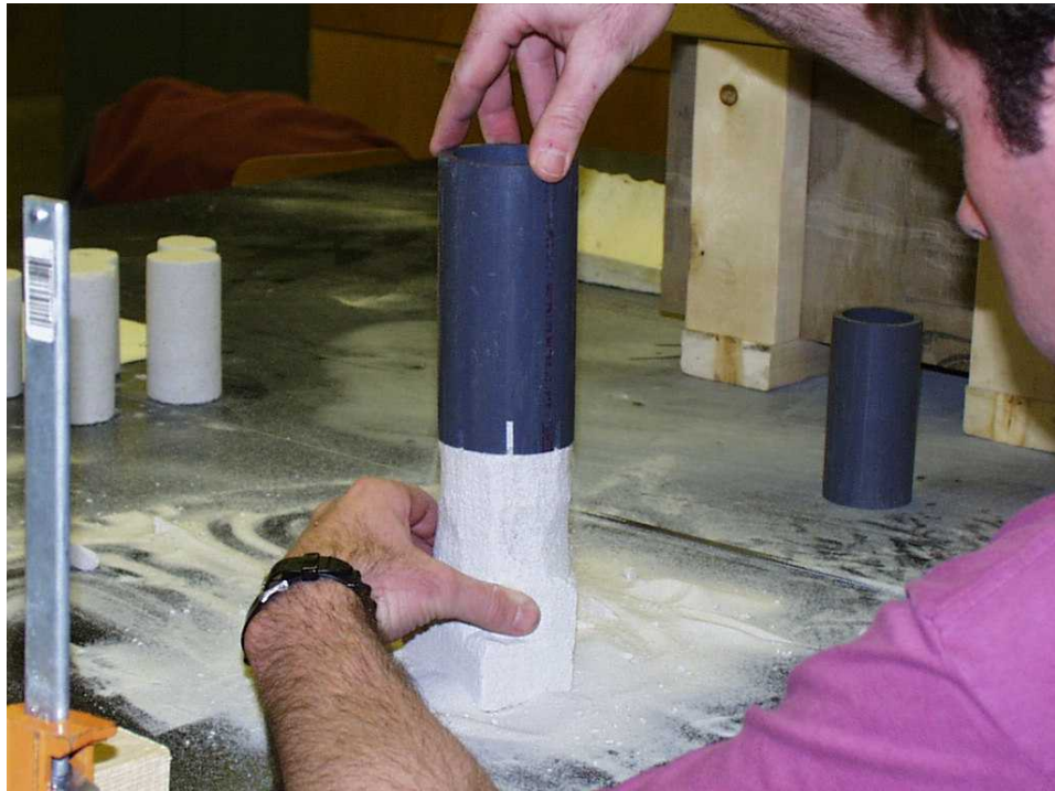
Figure 3-26: Coring the sample. This was done by rotating the PVC with slight downward pressure. The teeth cutting into the pipe are clearly visible.
