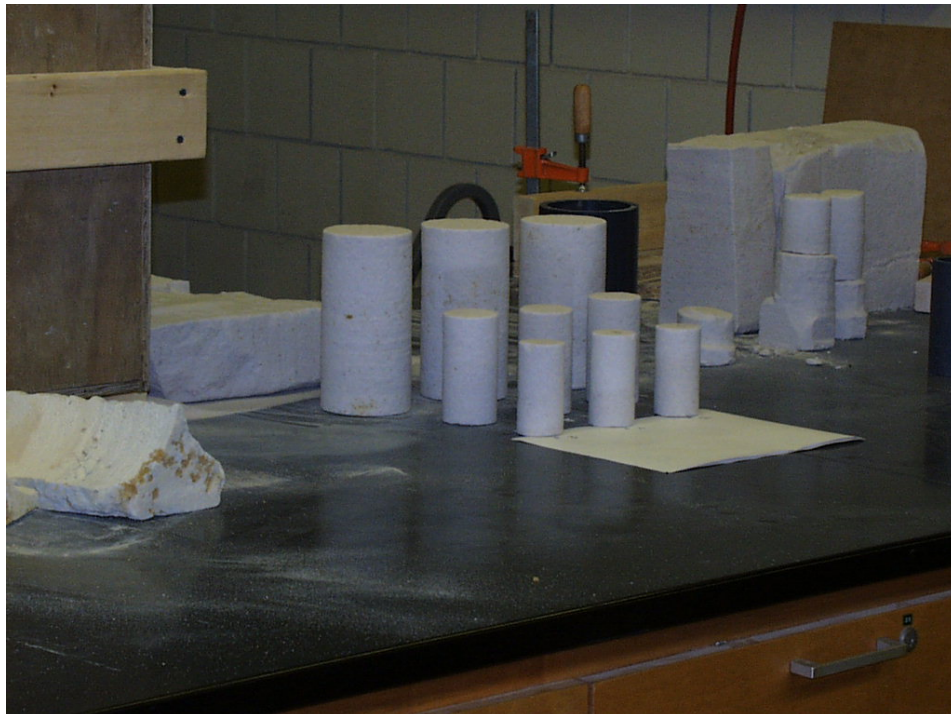
Figure 3-22: Finished St. Peter sandstone samples for uniaxial testing.
