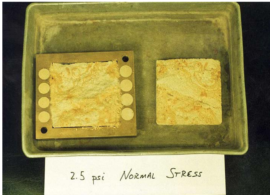
Figure 3-12: St. Peter sandstone sheared at 19 kPa normal stress showing considerable topographic relief in the shear zone.
