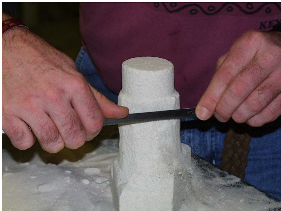
Figure 3-25: Trimming samples for coring.
