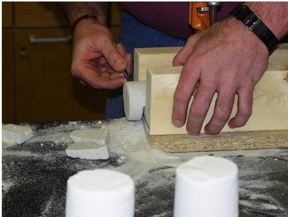
Figure 3-27: Squaring ends of the cores. Cores were squared to within 0.5mm on the ends.
