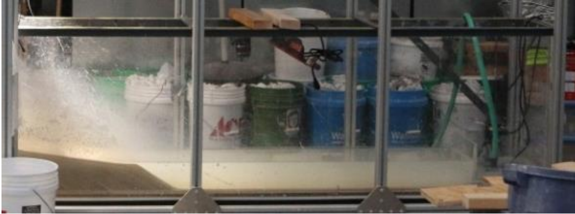
Figure 4.5. Side view of the depositional basin during Run 2. A delta has formed on the left side of the flume, where sediment and water from the drainage basin enters. A camera and a light source sit directly above the flume and record shoreline position through time. A weir on the far end of the flume sets sea-level and creates a reservoir on the right side of it. A pump drains the reservoir, sending water to the same drain that empties the source terrane.
