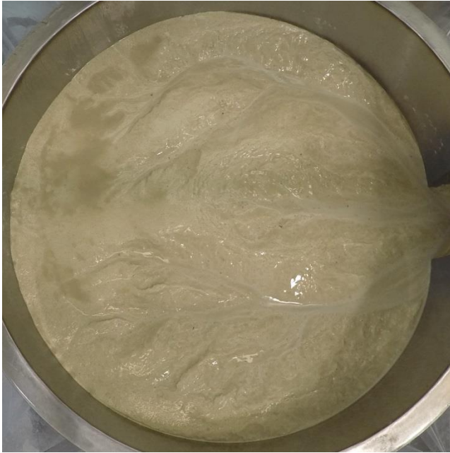
Figure 5.14. GoPro imagery of the source terrane roughly 10 hours into Run 3. While there was less relief than expected, the terrane did develop a dendritic network of self-formed channels.
