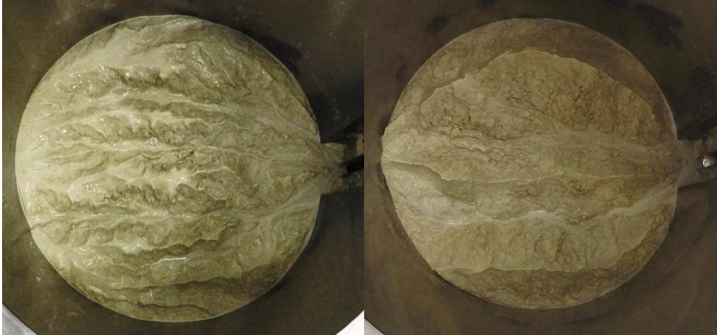
Figure 4.4. A view inside the drainage basin. Both images were taken by a GoPro camera during Run 2. The terranes slope towards the outlet located on the right side of both images. Note the slot on the right side. A stainless steel dam sets base level at the slot/outlet.
