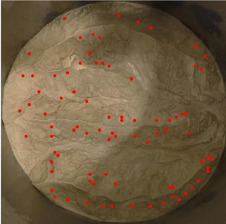
Figure 5.11. Landslide count at high uplift (83 in 30 minutes); red dots denote locations of landslides, which are distributed relatively uniformly along the lengths of ridges.
