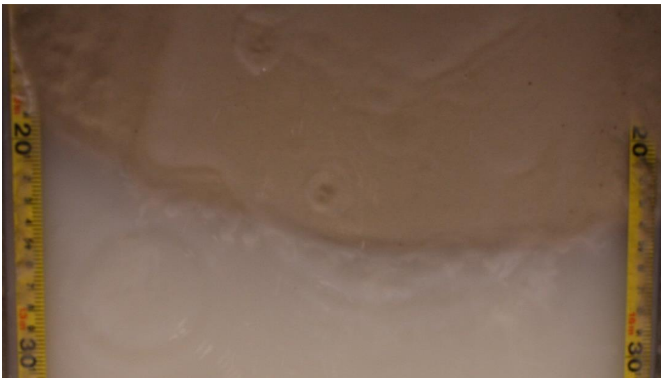
Figure 4.6. Image of fluvio-deltaic shoreline in experimental system. Topset of sandy delta is located towards the top of the image; the angle-of-repose delta foreset extends seaward of the shoreline, beneath the milky-colored free surface. Milky color of the ‘ocean’ is a result of suspended clay. Measuring tape stretched out directly above sea-level, on the inside of the flume walls provide spatial reference. Due to channel migration
