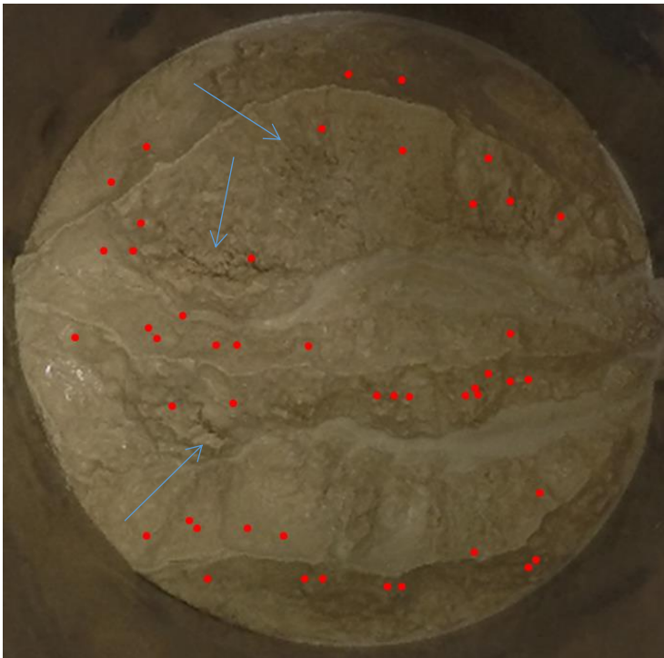
Figure 5.12: Landslide count at intermediate uplift rate (47 landslides). Light blue arrows point to ‘ravine-like’ features that formed during this phase of landscape response.
