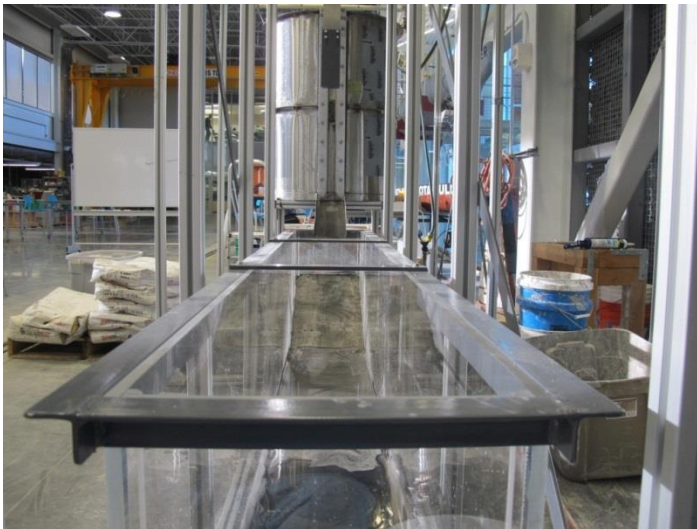
Figure 4.2. A view from the far end of the sink terrane (sedimentary basin), looking towards the source terrane (drainage basin). Sediment and water exit through the slot running vertically down the center of the source terrane as a metal dam is slowly lowered (simulating base level fall/tectonic uplift). All sediment and water travel down a stainless
