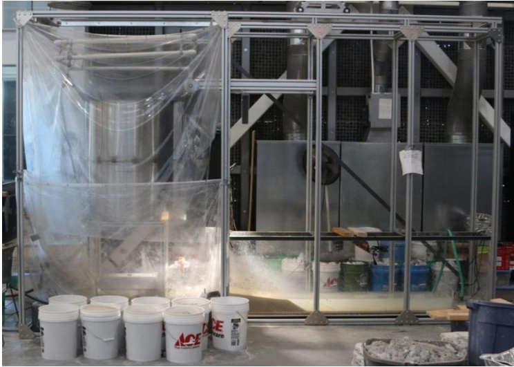
Figure 4.1. Source to sink experimental apparatus. The source terrane (left side of the image) is located in a stainless steel drum. PVC misters are located directly above the source terrane. Shower curtains are used to contain water and funnel it into a drain located below the source. The sink terrane (right side of the image) is essentially a plastic flume with metal supports to maintain its structure. Note the delta and ‘sea level’ inside the flume. Sea level is set by a weir found at the far end of the flume. An aluminum structure encases the entire apparatus. On top of the structure is a track system, on which a motorized cart carrying a Lidar scanner is utilized. The scanner has the ability to measure surface topography of both the source and sink terranes.
