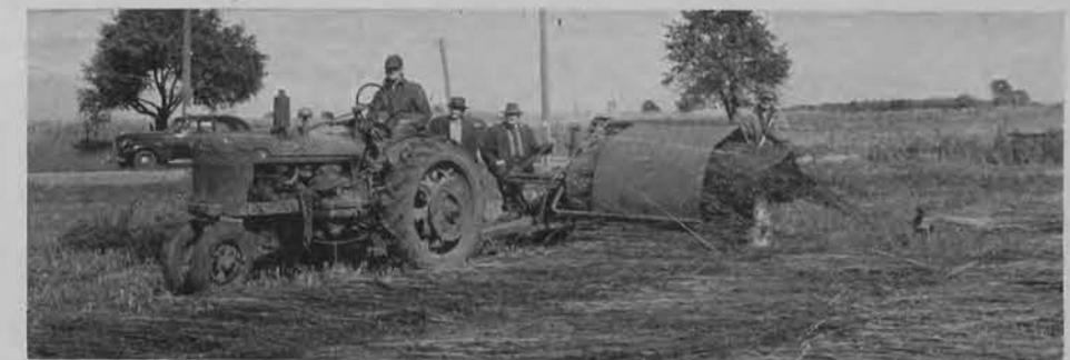
FIG. 2. This machine picks up and binds the hemp straw.
