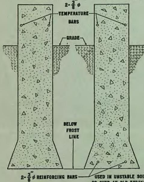
CRACKS APPEAR IN MANY FOUNDATIONS AT DOORWAYS AND OVER THE DOORS. THESE CRACKS MAY BE DUE TO FROST HEAVING THE FOUNDATION UNEQUALLY. REINFORCING BARS AS SHOWN WILL HELP TO HOLD THE FOUNDATION TOGETHER AS ONE UNIT.
