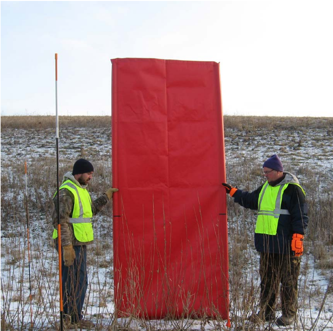
Figure 1.2 Using a large red backdrop to assess porosity in shrub-willow living snow fences.
