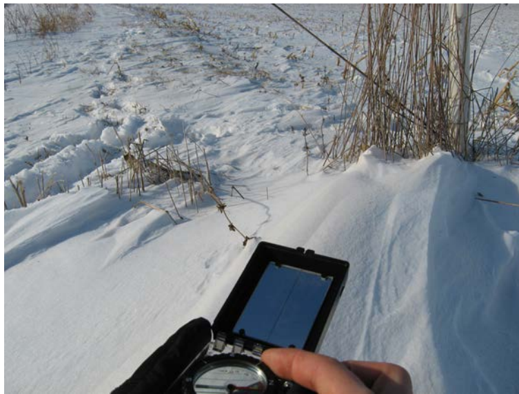
Figure A-1 Field-based method for determining direction of prevailing snow transport by measuring streamlined snowdrift orientation using a compass.
