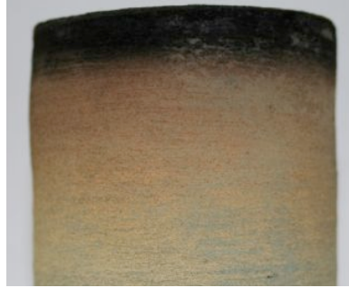
Figure 1.1: Image of a core of PICA material taken from the Stardust sample return vehicle [4].
