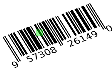
Figure 2.1: g_{ij} : intensity at the ij^{th} pixel (shown in green) is the average intensity over the pixel.
