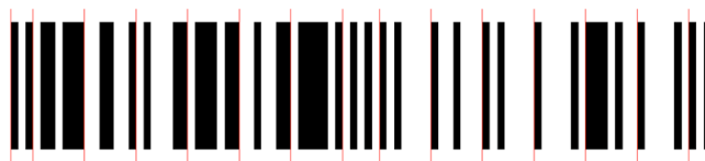
Figure 1.1: ‘814723686393’ encoded using UPC symbology. Each sequence for start, left digit, middle, right digit, and end is shown with divisions for identification ease.
