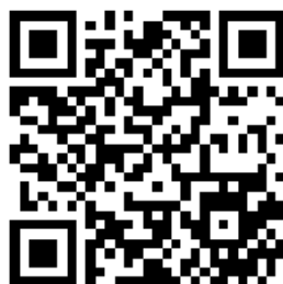
Figure 1.2: A sample Version 3 (29 by 29) QR Code encoding the link to the University of Minnesota SIAM Student Chapter homepage. This image was generated using www.qrstuff.com
