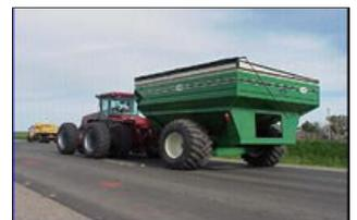
Testing is planned for two weeks in spring and in fall of each year under the national three-year pooled-fund study, "Effects of Husbandry 'Farm Equipment' on Pavement Performance, TPF-5(148)," The first spring tests, conducted from March 17 to March 26, included six pieces of farm equipment. Testing of 18 different types of equipment is planned. Private industries participating in the study are providing all test equipment.
