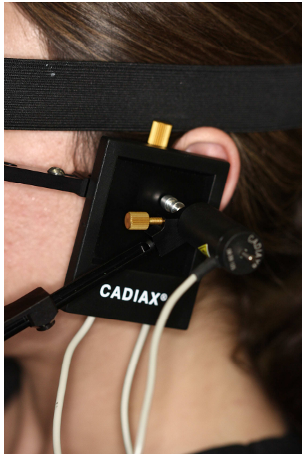
Figure 7. Recording plate and stylus positioned to record left condylar movements.
