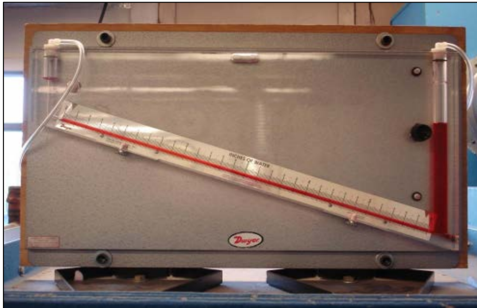
Figure 4-11: Dwyer inclined manometer
