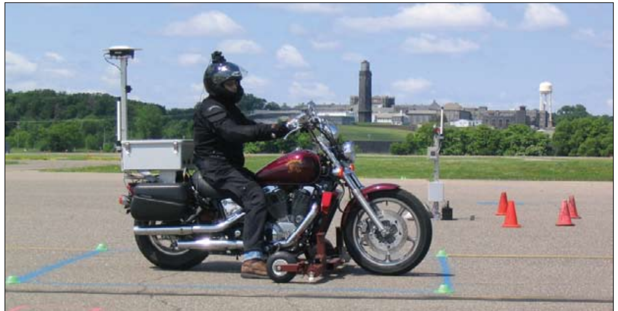
For their experiments, researchers added two outriggers that engage if the motorcycle tips during a test ride.
