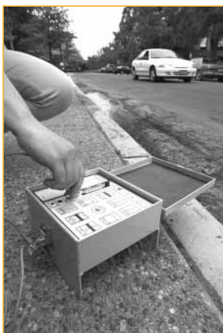
Researchers set up an automatic traffic recorder to collect data on individual vehicle speeds and headways.
