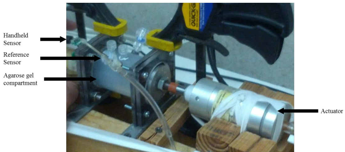
Figure 5-11: Experimental setup for measuring pressure with agarose gel compartment
