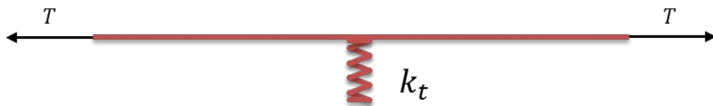
Figure 5-2: Model of the homogeneous model under a single transverse force
