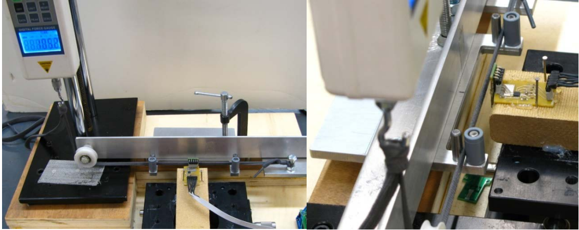
Figure 2-10: Photographs of the experimental setup for evaluating the sensor performance
