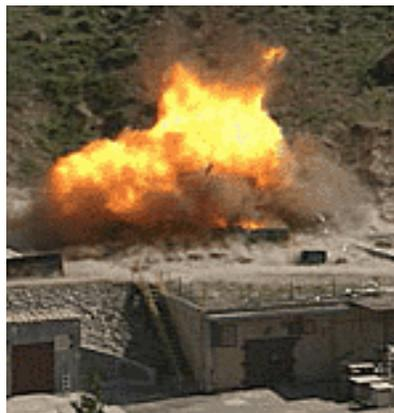
*Transient fields approaching 1000 tesla are generated by explosive compression of magnetic flux at the National High Magnetic Field Lab in Los Alamos.*
