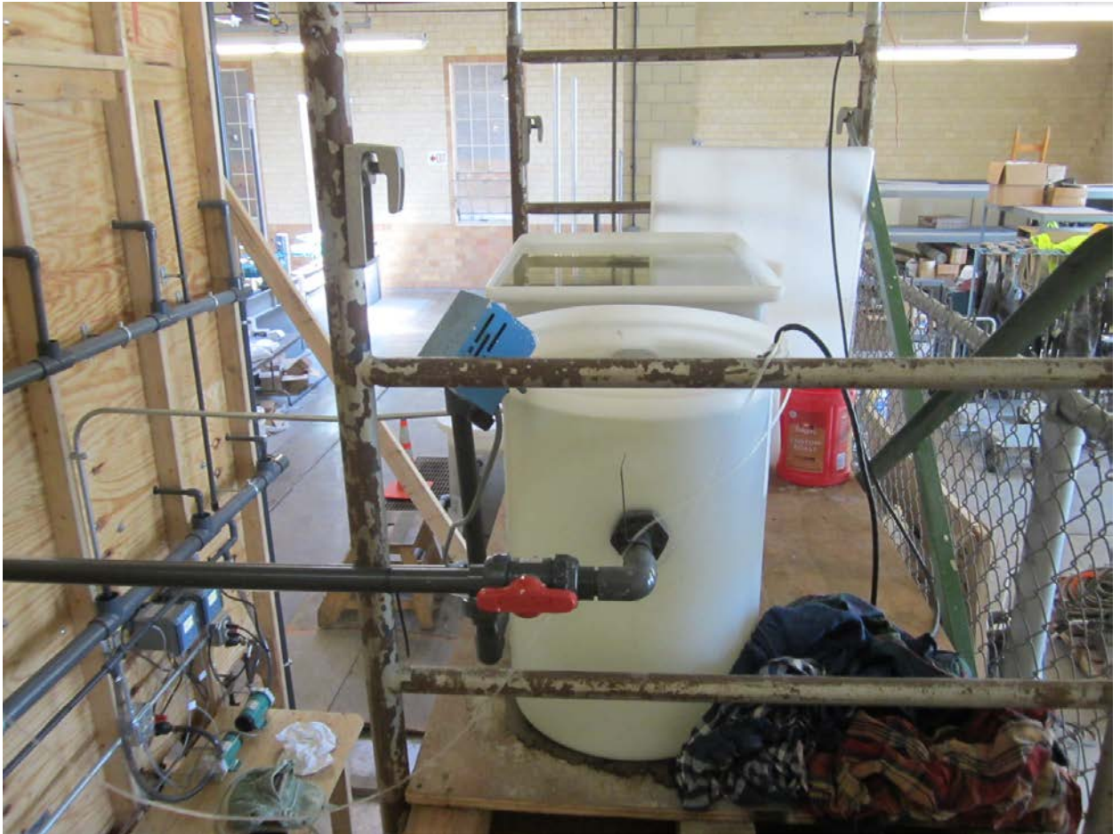
Figure D.4. Photo of the pilot-scale set-up rectangular settling tank and the circular overflow tank with mechanical mixer at MWTDS.
