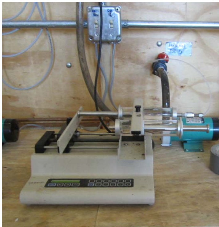
Figure D.5. Photo of the syringe pump used to dose geosmin into the pilot-scale set-up at MWTDS.
