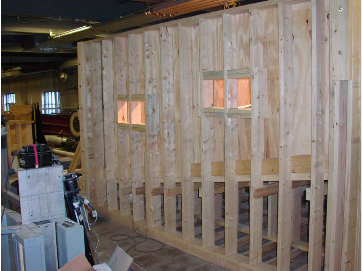
Figure 2.3. The basin test-stand made of lumber and plywood.
