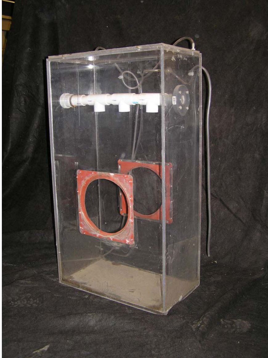
Figure 2.5. The flow-capturing apparatus to measure the flow rate out of two rings of orifices.
