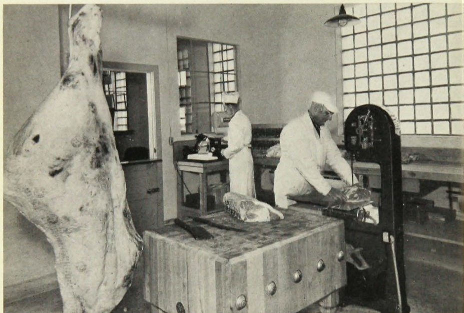
FIG. 5. THE POWER SAW SPEEDS UP MEAT CUTTING
