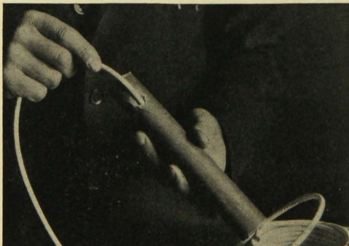
Fig. 5. The cap is completely hidden in the stick of dynamite.
