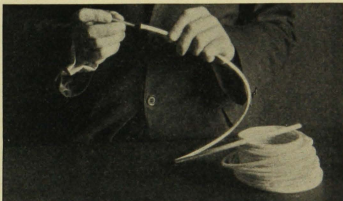
Fig. 2. If the end of the fuse has been cut off squarely, it is easily inserted into the cap.
