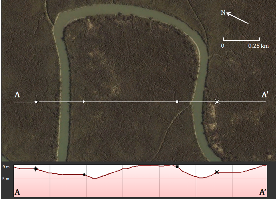
Figure 3.3: Elevation profile across an unnumbered channel. Google Earth imagery dated 1/10/07. Centered at 21.869049°N, 89.391796°E. Flood flow is from right side of page to left, ebb flow from left side of page to right. Notice the near-absence of topographic expression of the channel in the left portion of the cross section. Vertical scale is nonlinear.
