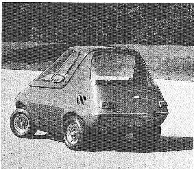
The 512 electric car. Built on a 52-inch wheelbase, it is 86.3 inches long. The 1,250-pound car is operated by an 84-volt power battery pack and has a 12-volt battery for accessories.
