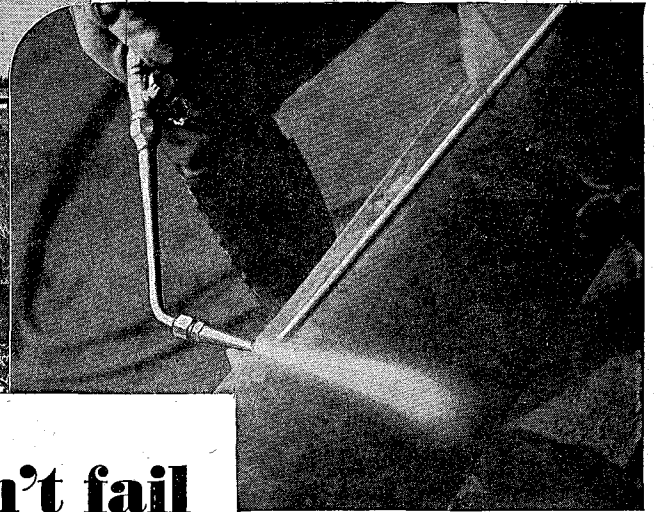
Two 10-in., one 14-in., and one 6-in. lines were laid on this trestle. Insert shows close-up of Multi-Flame Lindeweld Head in action.
