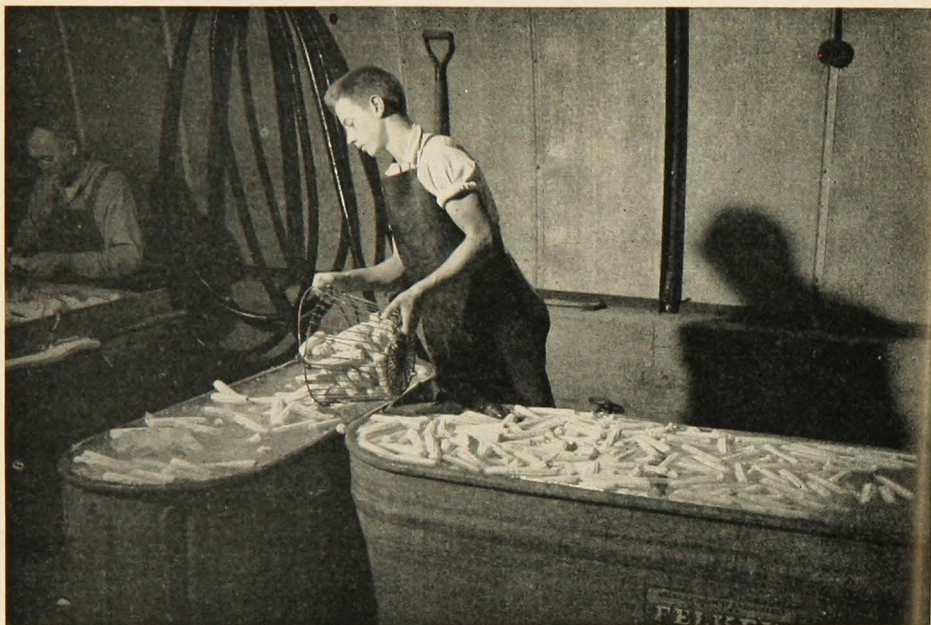
FIG. 1. Transferring corn from the initial cooling and washing tank (tank 1) to the iced tank 2. The sizing and packaging table is at the left background (1950).
