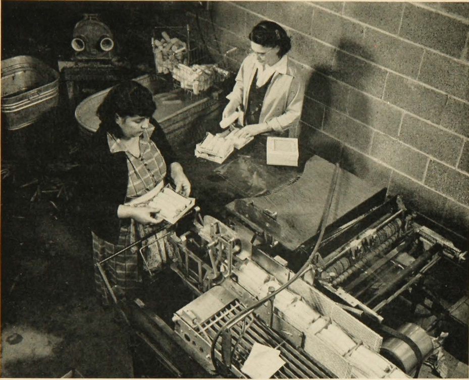
FIG. 12. Semi-automatic overwrap machine in operation. The ears are packed in a tray and overwrapped with perforated cellophane.
