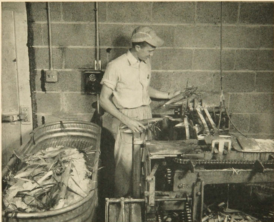
FIG. 10. Single-row Peerless corn husker cutting shank and removing husks. The operation requires a man to feed the husker from the tank. The husked corn is caught in a tub at the end of the husker.
