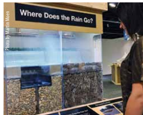
Pavers that let water through rather than run off the surface can retain more water on the landscape and lessen the impact of significant rainfall events.
