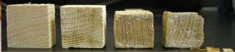
As brown rot progresses, wood retains its shape, but as the cellulose is removed the lignin shell loses strength and mass.
