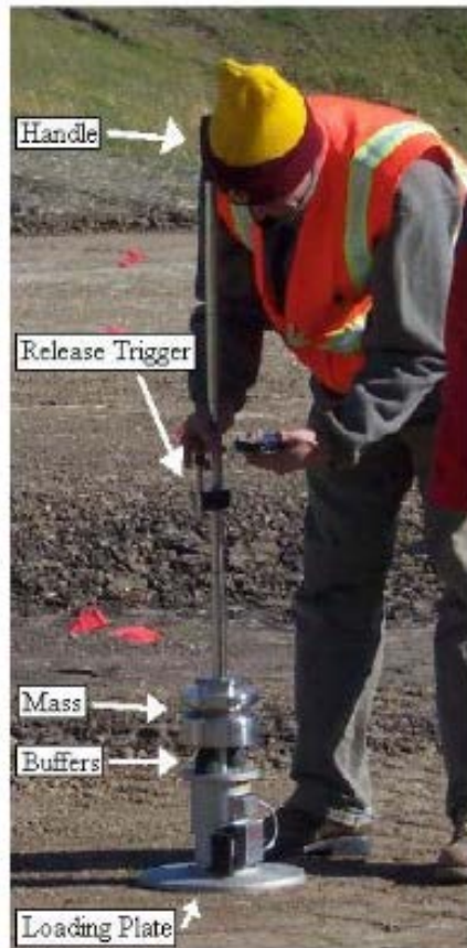
Figure 2: Photograph of the Light weight deflectometer (LWD) in the field (Seikmeier et al. [4]).
