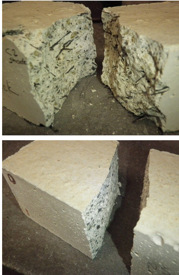
Figure 62: Needles Shown after Firing 304 (Left) 406 (Right)
