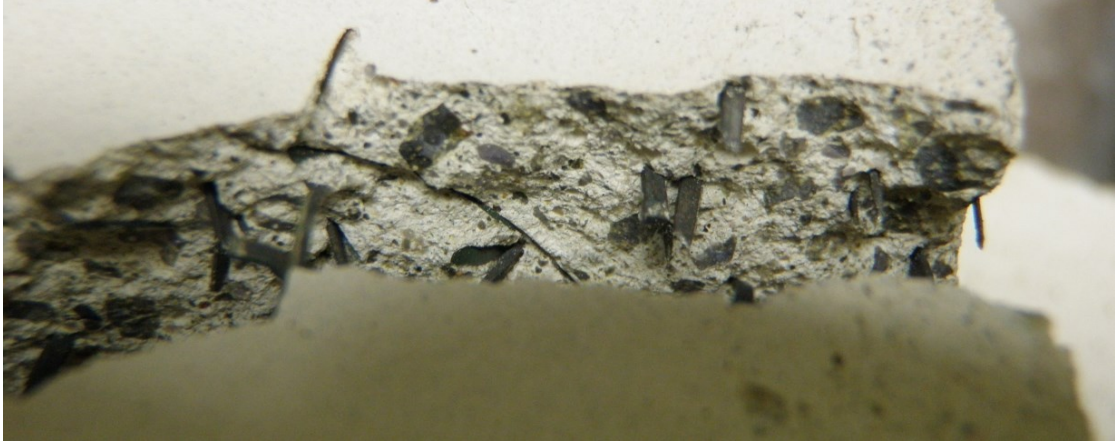
Figure 50: CMOR Beam Failure Showing Broken Needles
