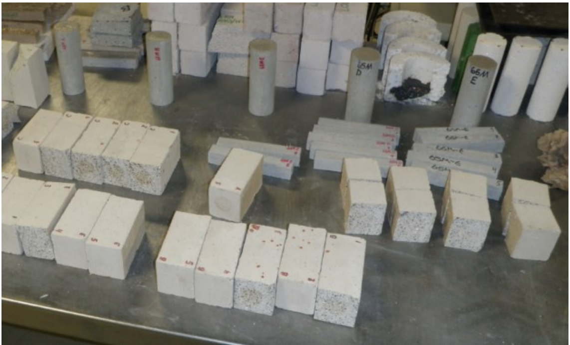
Figure 25: Thermal Shock and Thermal Dilation Test Samples
