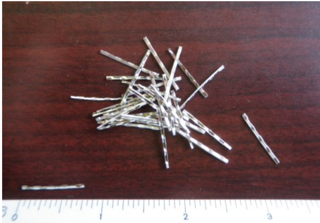
Figure 22: Typical Stainless Steel Needle \frac{3}{4} inch Long
