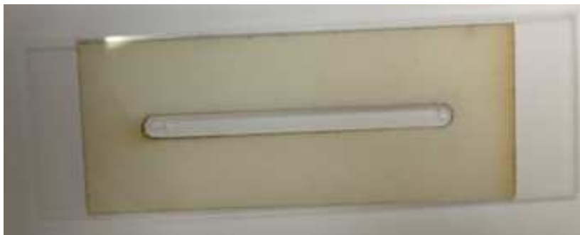
Fig. 5.4. Photographic image of the micro-fluidic channel used for high speed experiments to observe the rotation of the cell body. A 400 \mu\text{m} thick silicon shim is sandwiched between a glass slide and a thin cover slip (100 \mu\text{m} ).
