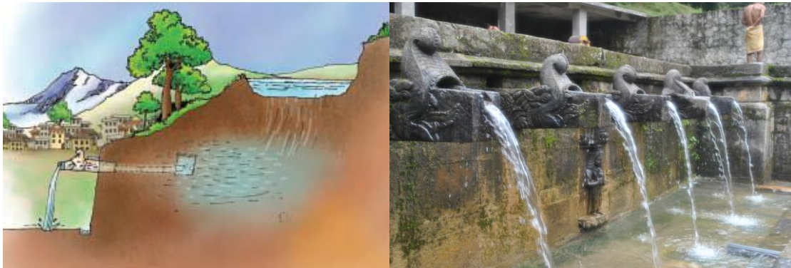
Figure 17 Traditional water supply system in Kathmandu Valley
