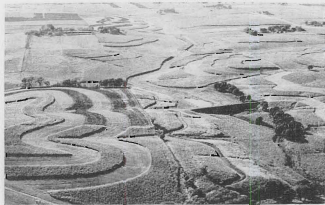
This is an air view of the detention dam and conservation practices in the East Willow Watershed Project in Fillmore County. The reservoir will store 202 acre-feet of floodwater, or 1.2 inches of runoff from the 1,980-acre watershed. The dam is 32 feet high and reduces the flood flow 71 percent.
