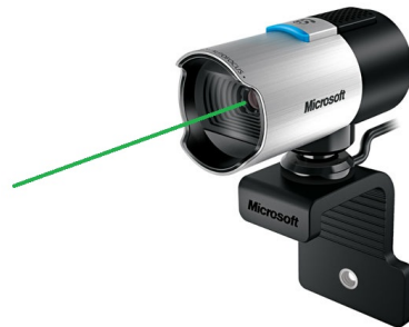
Figure 3.4: Microsoft Lifecam Studio Webcam, the optical axis is indicated in green.
