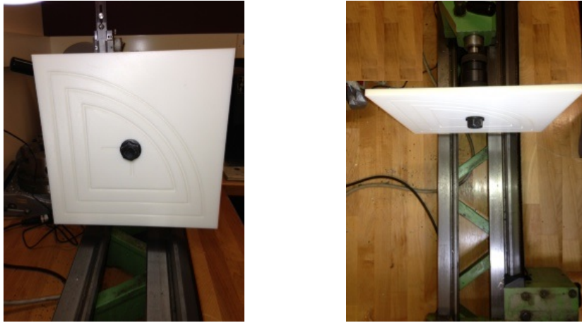
Figure 6.22: The trajectory board positioned in the lathe jig.
