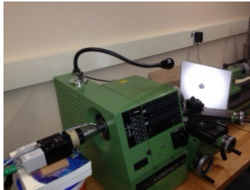
Figure 6.6: The endoscope calibration setup using a machinist's lathe.
