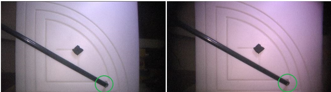
Figure 6.21: The tool tip is held still while the tracking algorithm is performed for noise characterization.
