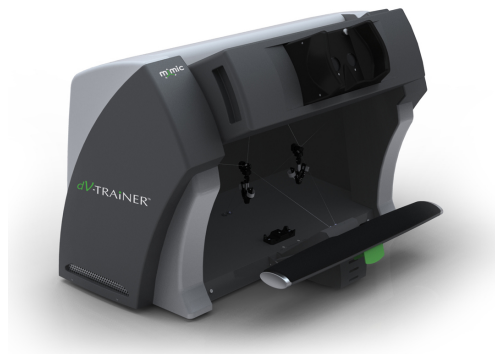
Figure 2.4: The MdVT virtual reality da Vinci simulator. Source: Mimic Technologies (Seattle, WA)
