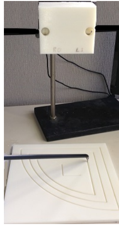
Figure 5.5: The stereo camera is placed above known trajectory.
