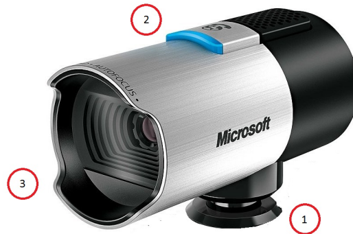
Figure 3.34: USB cable housing (1), top microphone(2), and lenses guard (3).
