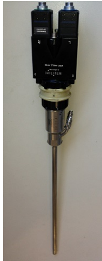
Figure 3.39: The da Vinci camera unit and Endoscope.
