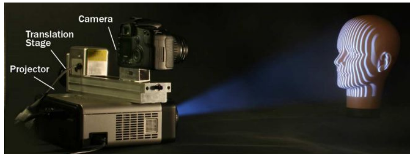
Figure 2.23: Basic Light-Stripping setup. [60]
