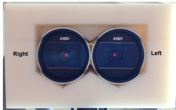
Figure 3.9: The stereo camera setup. The right and left cameras are labeled, seemingly in reverse since the cameras are pictured from the front. (See section 3.7 for details.)
