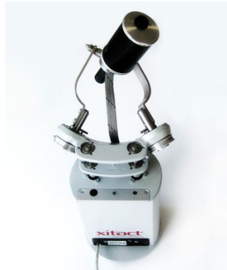
Figure 2.10: Tracking mechanism on the Xitact ITP. Source: Mentice AB (Gothenburg, Sweden)
