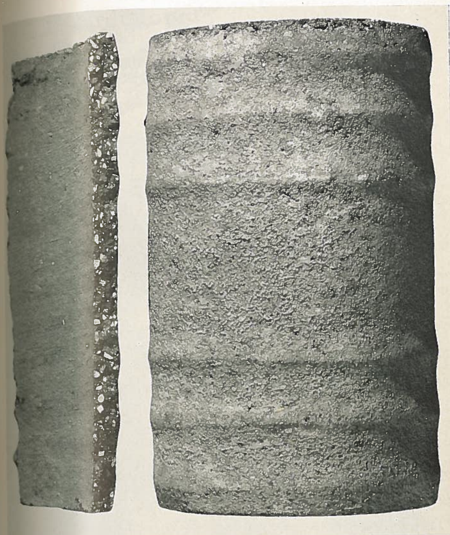
Fig. 1. Six-inch drain tile of good quality.
