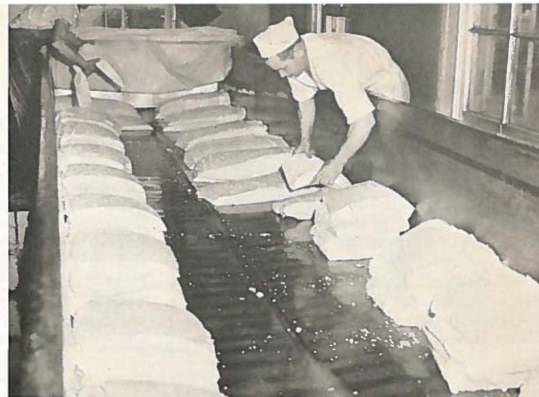
FIG. 3. Cheddaring is one of the stages in the manufacture of cheese.
