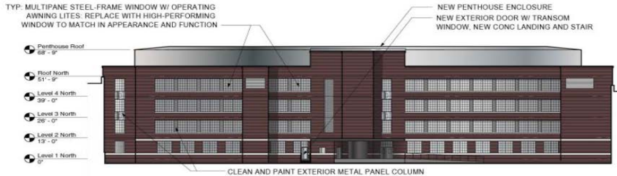
ELEVATION C: SOUTH FACADE OF NORTH WING
