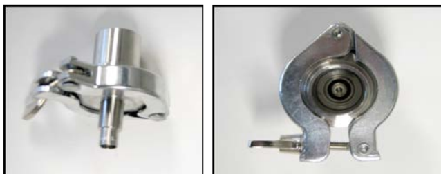
Figure 6.2. Coaxial sensor constructed from stainless steel vacuum feedthroughs.
