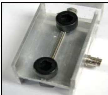
Figure 6.12. Single threaded sensor, 3.5" threaded stainless steel hot electrode in an aluminum U-channel ground. Packing tape used in-between the electrodes as the dielectric.
