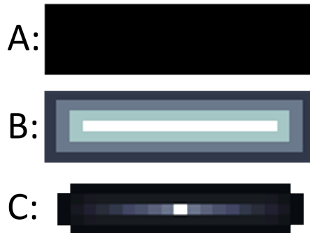
Figure 7.3: Shown here is a schematic representation of a binary cross-section ‘A’. This cross-section was subjected to both the distance map computation ‘B’, and calculation of the medialness function ‘C’. The distance map will not distinguish an exact center for elliptical cross-sections as a number of voxels can have the same value along the long-axis. As illustrated, the medialness measure computed from the GVF field allows definition of an objects center for elliptical cross-sections. This is important as vessel cross-sections are most frequently elliptical in nature.
