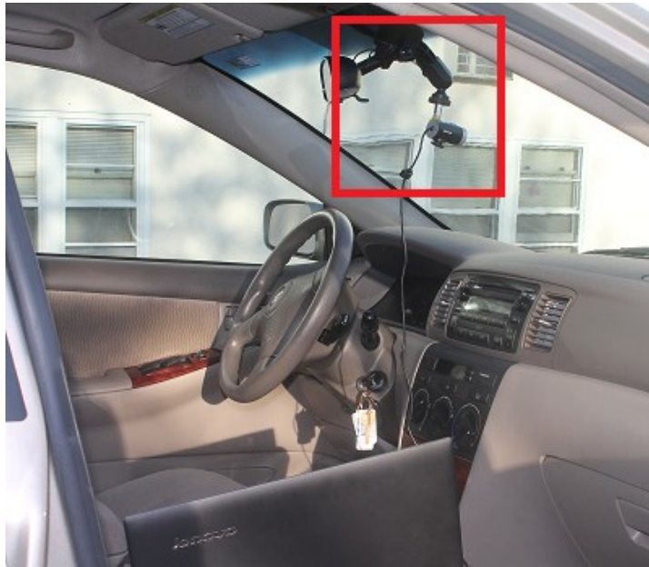
Figure 4.2: Camera installed in the vehicle with the help of a suction cup
